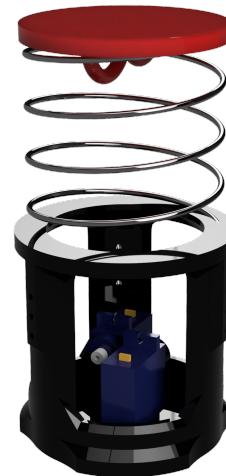
Fig. 11. Single spring release mechanism 3D prototype model.
