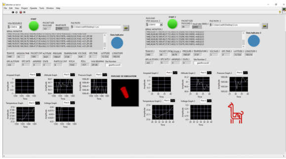
Fig. 14. LabVIEW interface for ground control station.
