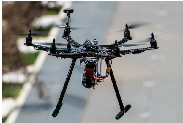
Fig. 2 Drone used to perform a communication test and a drop test
